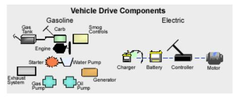
vehicle. The electric vehicle has several unique components that serve the same function as the more common components in a gasoline-powered vehicle.
